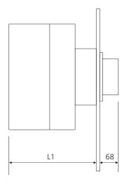
L1 = Mounting Depth L2/L3 = Panel Cut-out
