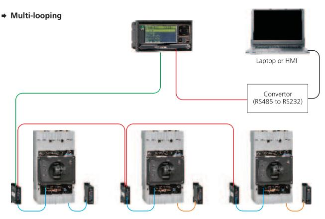
MODBUS Communication through MODBUS looping
